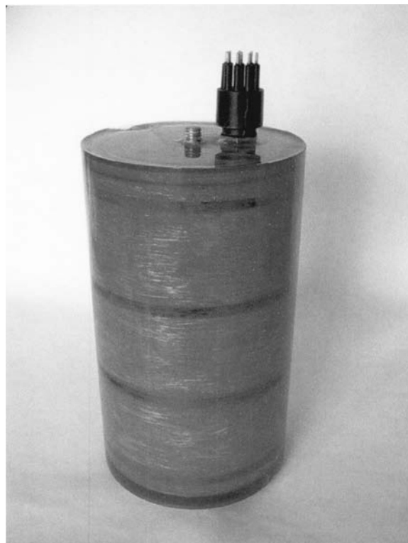
FIG. 8. A photograph of the encapsulated transducer with three piezoelectric cylinders and nine wire connector.
